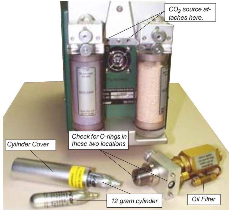
Figure 2-6. Location of external CO<sub>2</sub> source assembly.
