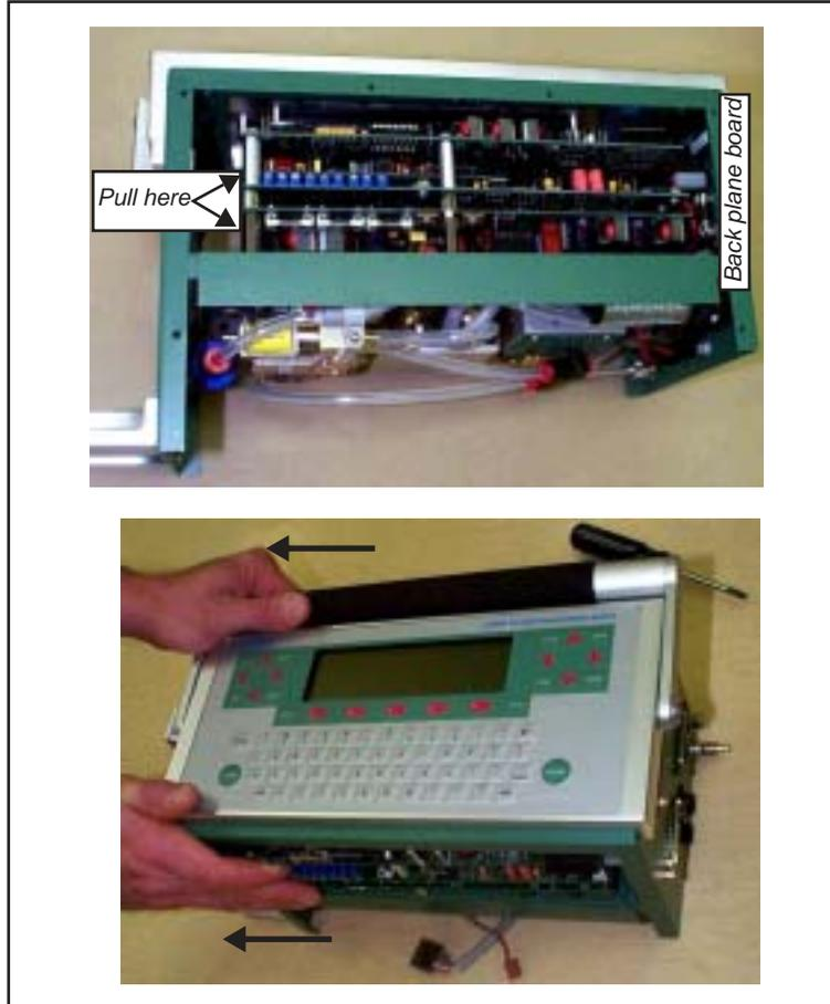
Figure 19-12. Unplug the board assembly from the back plane board by pulling (and rocking side to side gently) on the board stand-offs.
