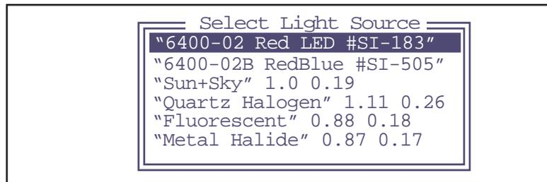
Figure 16-8. The light source menu includes standard sources, plus whatever 6400-02 and -02B sources have been installed.
