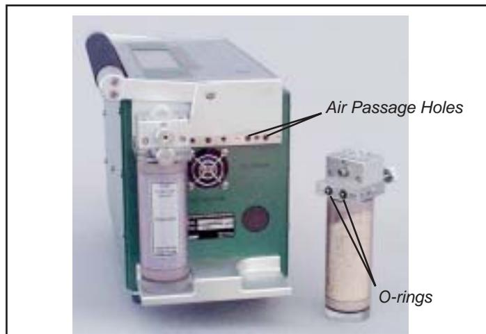
Figure 19-3. Each chemical tube has two air passage holes protected by O-rings.
