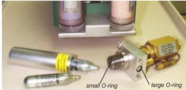
Figure 20-6. The CO<sub>2</sub> regulator's O-rings.
