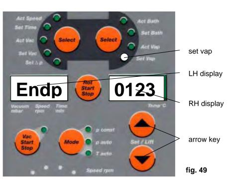
appears in the lefthand display; at this point select final pressure. Final pressure so selected appears in the righthand display.
