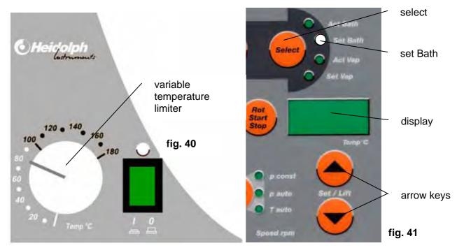
Select "Set Bath" with select key and set nominal temperature with arrow keys. Nominal temperature is displayed. After 5 seconds, display automatically returns to actual indication (Act Bath).
