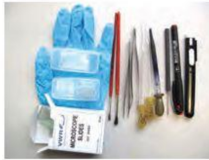
Fig. 4.2. Preparation tools: gloves, paint brushes, tweezers, pipettes, needle, paper knife, marker, slides and cover glasses.
