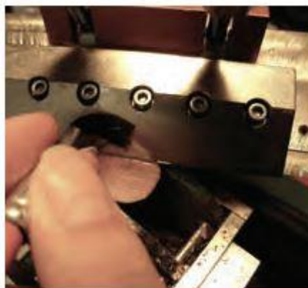
Fig. 3.72. Keeping the section flat with a painting brush on the blade.
