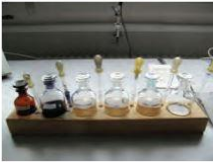
Fig. 4.1. Holder with chemicals for preparation of permanent slides. It contains dyes, ethanol and xylene and corresponding pipettes.
