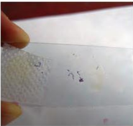
Fig. 4.33. The small sections are trapped in the viscous Canada balsam.
