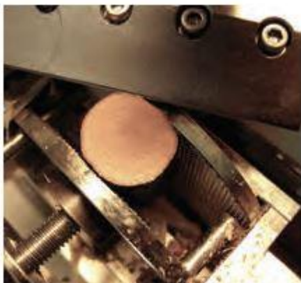
Fig. 3.70. Position of the pulling angle of the blade in relation to the object. The optimum angle of the knife is around 45 degrees, but depending on the species of your sample and the desired quality of your section, this angle should be adjusted until an optimal section is achieved.
