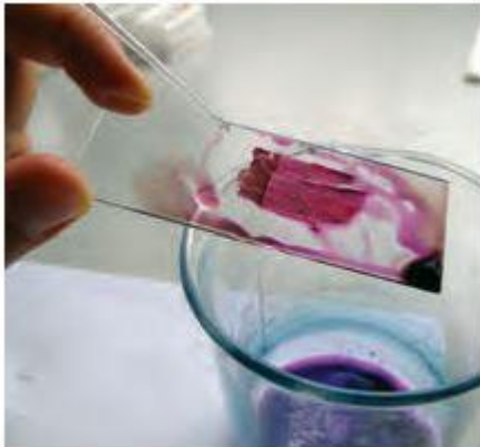
Fig. 4.28. Dehydration of a section of wood.
