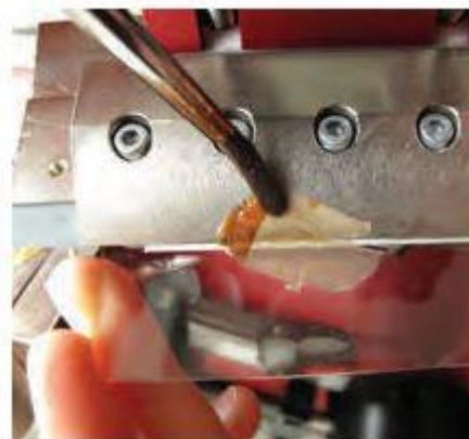
Fig. 3.73. 'Swimming' or gliding a section from the blade onto the glass slide.
