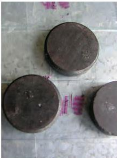
Fig. 4.37. Slides on an iron plate between plastic strips, and weighed down with magnets.
