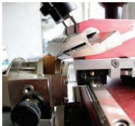
Fig. 3.71. Position of the angle of inclination of the blade in relation to the object. For hard woods, e.g., tropical woods the incline should be fairly steep. In soft material, e.g., archeological wet wood, the incline should be as flat as possible.
