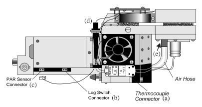
Figure 28-6. Preparing to remove the standard leaf chamber.
