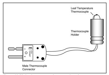
Figure 19-22. Leaf temperature thermocouple and connector.
