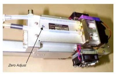
Figure 18-9. Location of the leaf temperature zero adjustment screw.
