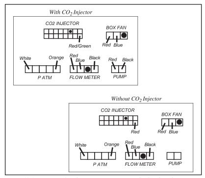
Figure 19-15. Diagram for plugging in connectors to the flow board. On instruments that do not have a  $CO_2$  injector, the pump connector is left empty. The pump plugs in to the  $CO_2$  injector connector, instead.
