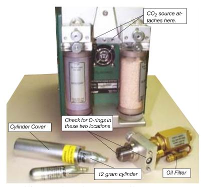
Figure 2-6. Location of external  $CO_2$  source assembly.
