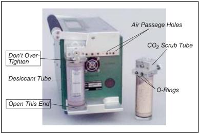
Figure 2-1. Desiccant and CO<sub>2</sub> scrubber tubes.
