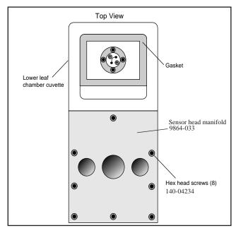
Figure 19-32. Remove the optical bench cover (leave the chamber bottom attached) by removing the 8 screws in the manifold.
