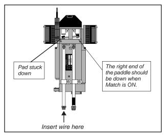
Figure 19-26. If a pad sticks preventing the match valve from operating, insert a thin wire as shown and pop the pad free.
