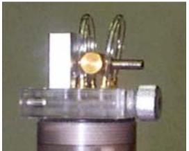
If the small tubing remains compressed long enough (especially in hot weather), they can seal closed. If that is the case, replace them. Also, check carefully in the hose barbs and air passages in the clear plastic base of the assembly for any debris that might be lodged there, blocking the flow.
