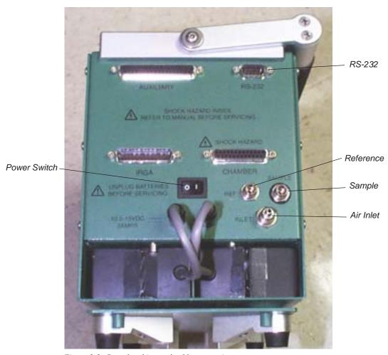
Figure 2-2. Console tubing and cable connections.
