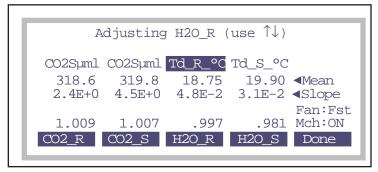
Figure 18-6. Adjusting the  $H_2O$  span. Adjust until the displayed dewpoint value matches what the LI-610 is set to.
