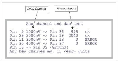
Figure 21-1. The AuxDacTest display. Press any key to change the mV settings on the DACs.. The change cycles between 1-2-3-4 V, 4-3-2-1 V, and 0-0-0-0 V. If the DAC output and the analog input are within 50mV, then the status will show "ok". Otherwise, it will show "ERROR".
