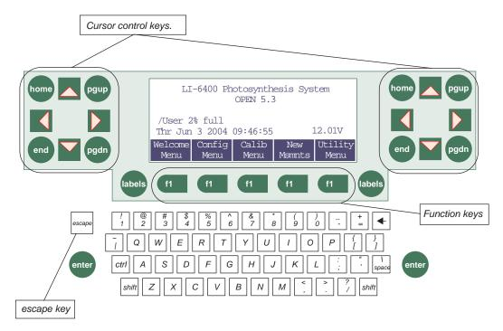
Figure 3-1. The LI-6400 keypad. The cursor control keys, labels, and enter are paired to facilitate access with either hand.
