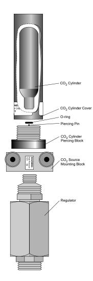
The optional 6400-01 CO $_2$  Injector consists of a controller that is factory installed within the LI-6400 console, and an external part that attaches between the chemical tubes on the end of the console. This external part can be either
