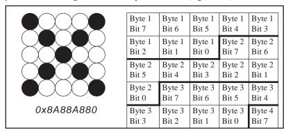
Figure 24-4. Relation between location in the 5x5 image and bits in the source Long. In the example on the left, the value 0x8A88A80 results in a 5x5 X image.
