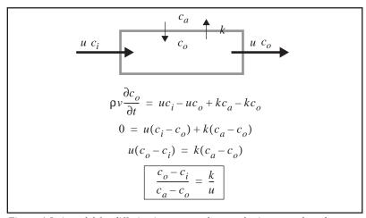
Figure 4-9. A model for diffusion in an open photosynthesis system, based on conservation of mass. The walls of the system have  $CO_2$  leak rate k (mol  $s^{-1}$ ). u is bulk flow rate (mol  $s^{-1}$ ), and  $c_i$ ,  $c_o$ , and  $c_a$  are incoming, outgoing, and ambient  $CO_2$  concentrations (mol mol<sup>-1</sup>). In steady state, the change of  $CO_2$  with time in the system is 0.
