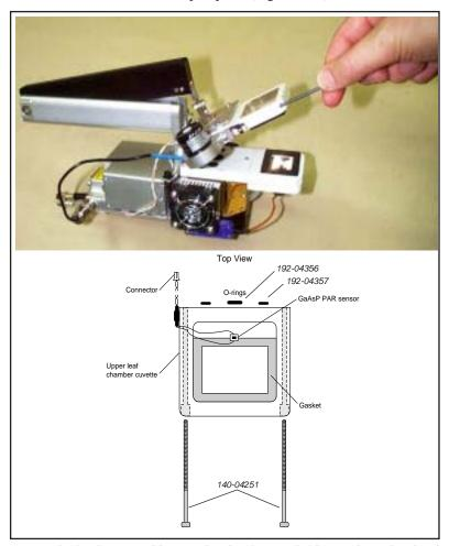
Figure 2-12. The top and bottom chamber lips are held on with two hex head bolts. Use the 3/32 inch hex key to loosen and tighten them.
