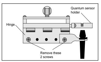
Figure 19-31. Remove the 2 screws shown.
