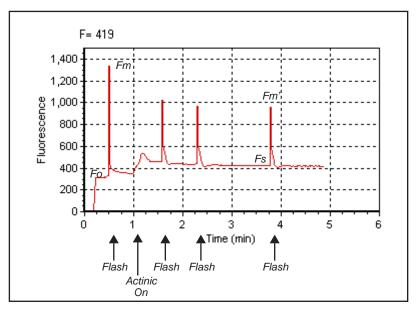
Figure 27-29. Fluorescence parameters of a light-adapted plant upon application of a saturation flash.
