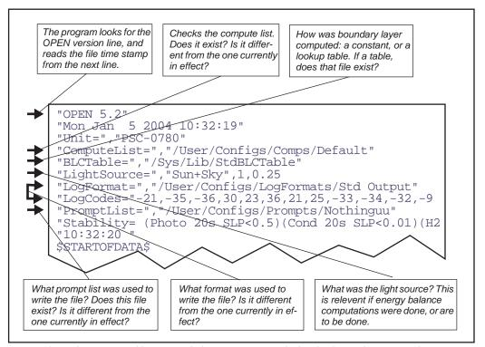
Figure 13-7. When a source file is opened, the program scans the header for configuration information.
