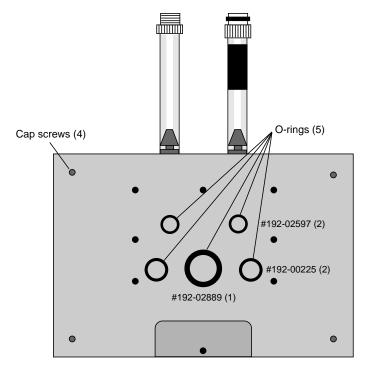
Figure 28-14. Location of the O-rings and cap screws.
