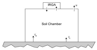
Figure 28-33. Schematic of the soil chamber. Soil evaporation  $f_w$  and soil CO2 flux  $f_c$  add mass to the chamber air, which is balanced by flow u (mixture of air, water, and CO<sub>2</sub>) out of the chamber.
