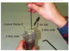
Using a 3/32 hex key, remove the three screws on each side of the assembly, and two of the four screws from the top. Leave the two top screws that are closest to the flow adjust bolt side (opposite the side where the nut was) of the assembly.
