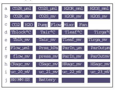
Figure 20-15. The diagnostic display map for New Measurements mode.
