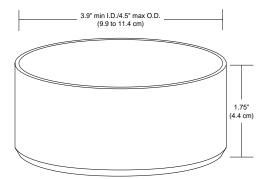
Figure 28-31. Soil collar dimensions.
