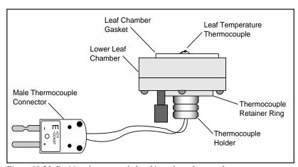
Figure 19-23. Position thermocouple bead just above foam gasket.
