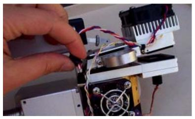
Figure 20-9. Unscrew the lamp connector to access the four wires. Caution - High Voltage.
