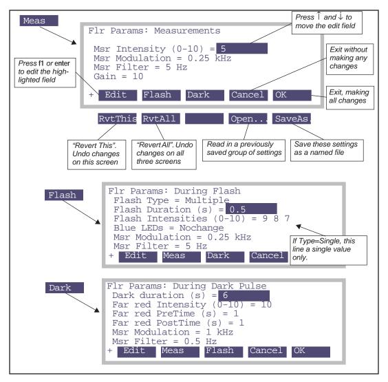
Figure 27-25. The Flr Editor, accessed by pressing f2 level 8. The editor is a dialog with three screens. Press Meas, Flash, and Dark to move between the screens.
