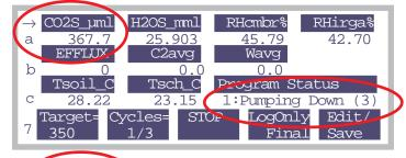
2. CO2S\_uml is now low enough, so the pump turns off. We are waiting for the value of CO2S\_uml to rise above Target - Delta, so the measurement can begin.
