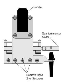
Figure 28-9. Remove the screws on the back side of the handle.
