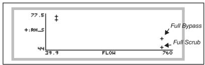
Figure 3-52. Sample humidity as a function of flow rate from Experiment #1.
