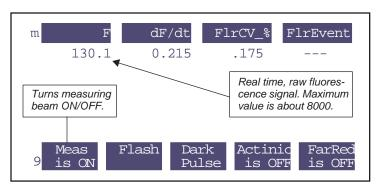
Figure 27-16. Basic fluorescence monitoring and control
