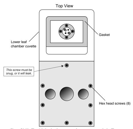
Figure 20-11. The eight hex head screws must be snug to prevent leaks. The top screw is extra important, however, because it passes through one of the air passages in the manifold, and there is just a metal-to-metal seal beneath the screw head.
