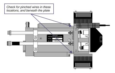
Figure 20-10. Check this metal cover to be sure that it is not pinching any of the wires that come out from beneath it, especially near the match valve.
