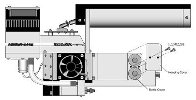
Figure 19-28. Remove the two screws that secure the housing cover.
