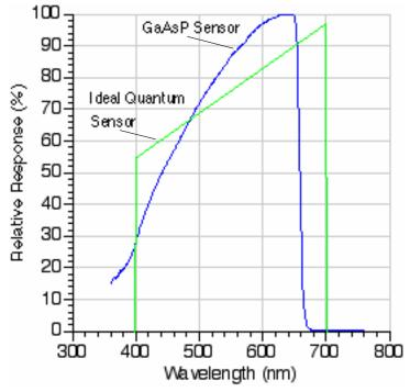
Figure 8-5. Spectral response of GaAsP sensor and ideal quantum response.
