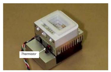
Figure 20-8. The temperature sensor in 6400-02B's.
