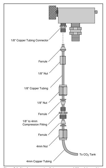
Figure 2-9. Use the compression fitting to connect 1/8" and 4mm tubing.
