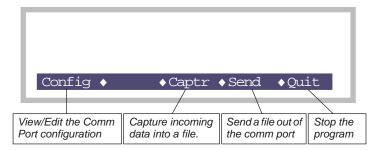
In file capture mode, the destination file is selected using the Standard File Dialog. While data is being captured, the display will show only a byte count of captured data, not the actual data.
