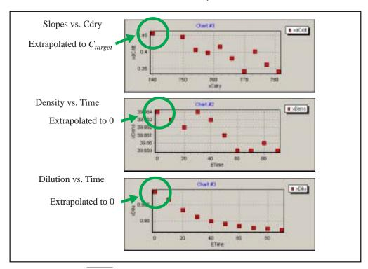
Figure 16-29. Plot of  $\frac{dC}{dt}$ ,  $\bar{\rho}$ , and  $\bar{D}$  from Figure 16-5. The circled points are the Mode 2 values.
