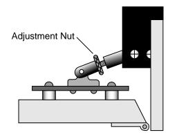
Figure 28-8. Turn the adjustment nut clockwise to remove.
