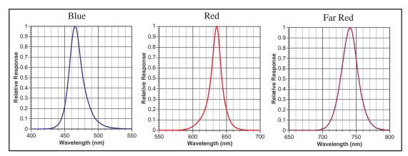
Figure 27-2. Relative spectral outputs of the three types of LEDs used in the LCF: a) Measuring and actinic, b) actinic and saturation flashes, c) far red.
