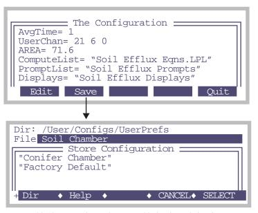
Figure 28-19. saving the configuration file for the soil chamber.
