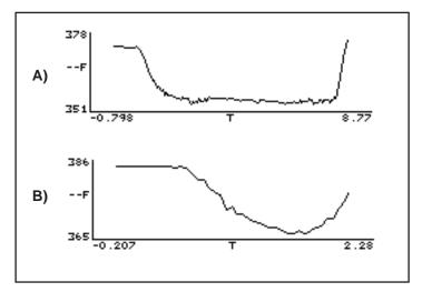
Figure 27-32. A) Example of a good dark curve: far red intensity and time were appropriate for the leaf material (notice the curve flattened before the actinic light was turned on). B) Example of a poor dark curve: far red intensity is not bright enough and time is too short to get a flat curve.
