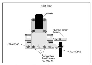
Figure 19-21. Remove the indicated screws.
