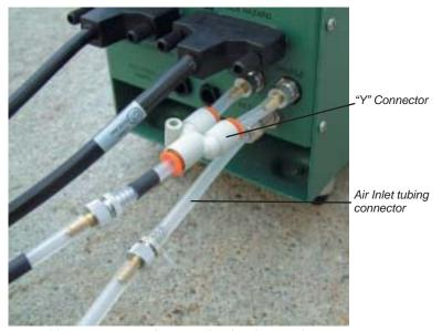
Figure 28-17. Connecting the sensor head to the console.
