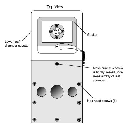
Figure 28-12. Remove the 8 hex head screws.
