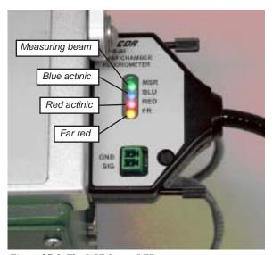
Figure 27-3. The LCF Status LEDs
