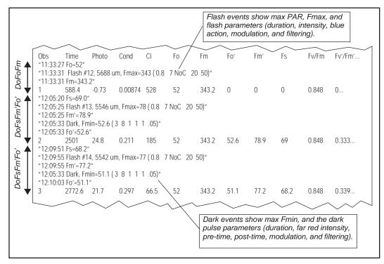
Figure 27-52. Sample lines from a data file showing remarks generated by fluorescent measurement events, and data records. At 11:33:27, a DoFoFm was performed, causing Fo to be set. A saturating flash was completed at 11:33:31, and the value of Fm set accordingly. A data record was then logged, using gas exchange data from 11:33:27. Observations 2 and 3 were each triggered by a DoFsFm'Fo' event.
