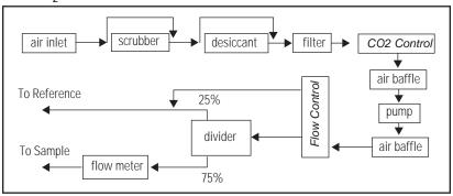
Figure 20-12. Flow schematic with and without the 6400-01  $CO_2$  Mixer. A more complete schematic is found in Figure 20-16 on page 20-46.
