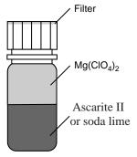
Figure 19-29. Fill the bottles with the CO<sub>2</sub> scrubber, followed by magnesium perchlorate.
