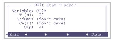
Figure 3-61. Editing an entry in the stability list. T is time period for the running computations, StdDev is standard deviation, CV(%) coefficient of variation, as percent, and Slp is slope (rate of change with time).
