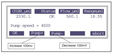
Figure 18-11. Pump speed is adjusted with the function keys, between 1000 mV and 5000 mV. Default pump speed is 4500 mV.
