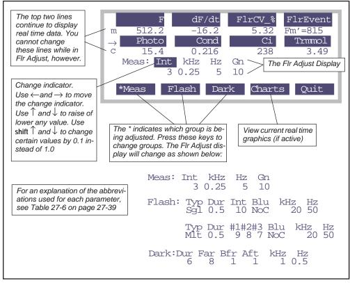
Figure 27-26. The Flr Adjust mode, allows any fluorescence parameter to be adjusted "on the fly" using only the arrow keys  $\leftarrow \uparrow \downarrow \rightarrow$ , without interrupting normal New Measurements operations. Pressing **shift**  $+ \uparrow or \downarrow$  increments the selected field by 0.1 rather than 1.0.
