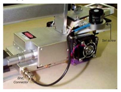
Figure 2-10. The external quantum sensor installed.
