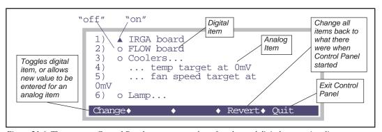
Figure 21-6. The program Control Panel presents a number of analog and digital outputs in a list.
