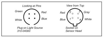
Figure 16-21. The pins that go into holes 1 and 2 are the ones to use for wiring a fan. Blue (1) is ground, Red (2) is power.
