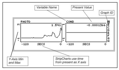
Figure 3-17. The default Real Time Graphics (RTG) display A in New Measurements mode shows photosynthesis and conductance.
