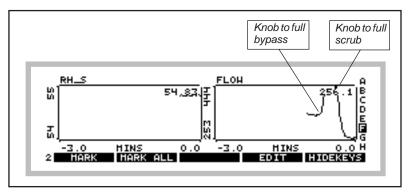
Figure 3-36. Flow increased when desiccant was put on full bypass, then dropped when desiccant was put on full scrub.
