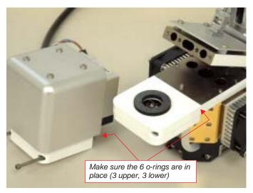
Figure 27-7. The LCF lower chamber attached, and the upper chamber ready.
