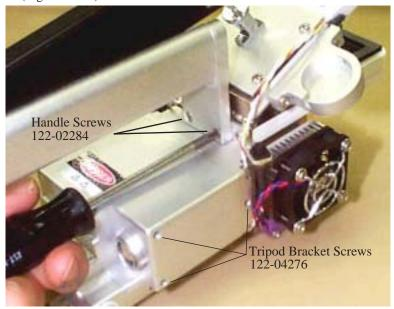
Figure 19-17. Keep the handle screws snug. Older units have three screws.
