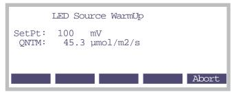
Figure 18-17. The calibration curve is generated automatically. SetPt is the command signal, and QNTM is the resulting PAR ( $\mu$ mol m<sup>-2</sup> s<sup>-1</sup>).
