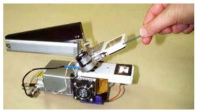
Figure 27-6. Remove the chamber top and bottom using a 3/32" hex key
