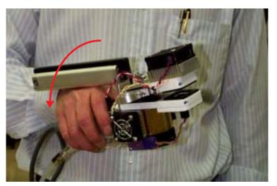
Figure 20-4. Grasp the IRGA as shown, then flick (abruptly turn) your wrist to try to start a stalled chopper motor.
