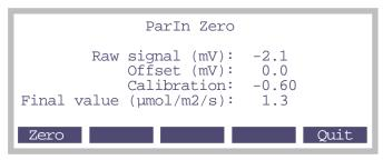
Figure 18-15. The program for zeroing the ParIn signal.
