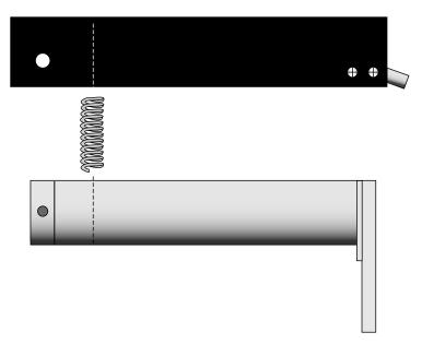
Figure 19-19. The latch return spring is in the rear of the handle. To access, remove the bolt in the rear that serves as a hinge.
