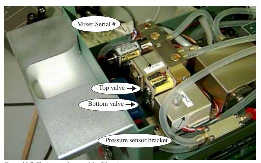
Figure 20-7. The in-console part of the CO<sub>2</sub> mixer.
