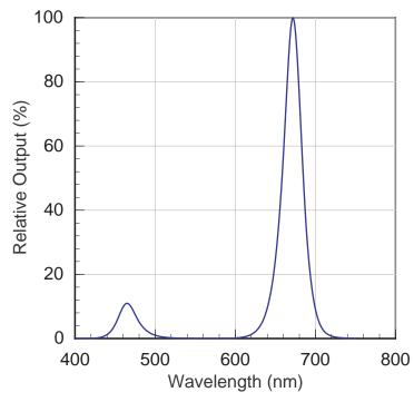
Figure 8-3. Typical output of a 6400-02B LED source at 25°C. (A 6400-02 source has the same red peak, but no blue peak.)
