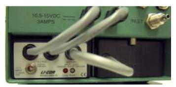
Figure 2-14. The 6400-70 AC Module fits in a battery compartment in the console. If you install a battery in the other compartment, and plug it into the module (as shown here), that battery will trickle charge, but more importantly, provide continued operation for 1-2 hours in the event of a mains power failure.
