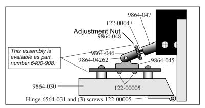
Figure 19-20. Unscrew leaf chamber adjustment nut.
