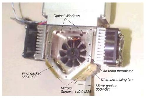
Figure 19-33. Clean the two optical windows.
