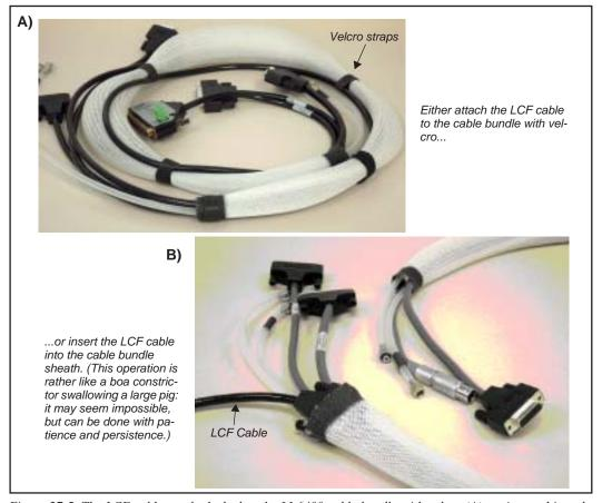
Figure 27-5. The LCF cable can be lashed to the LI-6400 cable bundle with velcro (A), or inserted into the bundle (B). If you choose to do the latter, insert the smaller connector into the console end of the bundle (the end with two 25 pin connectors) so it will come out at the sensor head end.
