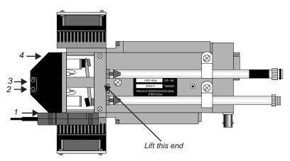
Figure 19-27. Remove the match valve cover by removing four screws, and lifting the cover from the indicated end.
