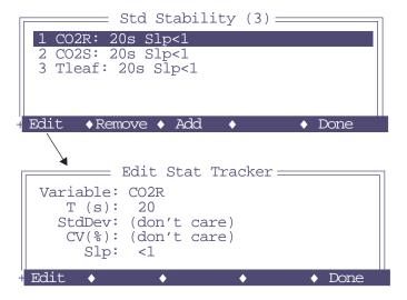
You can monitor some variables in New Measurements mode that indicate the state of system stability. In addition to this, statistical details can be viewed in a diagnostic screen, described in the next section.
