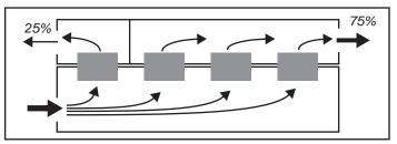
Figure 20-14. Schematic representation of the LI-6400's flow divider, that partitions flow to the sample and reference cells of the IRGA.
