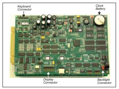
Figure 19-13. The PC boards out of the console. Digital board is the one shown.
