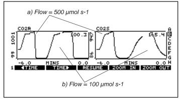
Figure 3-39. Controlling on reference  $CO_2$  concentration, with a closed, empty chamber. Note the slower response of the sample cell (due to its larger volume) is aggravated at lower flow rates. Note also the faster response when lowering  $CO_2$  than when raising it.
