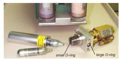
Figure 20-6. The  $CO_2$  regulator's O-rings.
