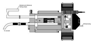
Figure 28-32. The "to chamber" line attached to the sensor head, for zeroing purposes.
