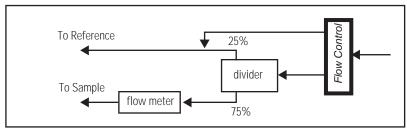
Figure 4-15. Flow schematic for units with a 6400-01  $CO_2$  mixer. Flow control is done with a diverter valve, and the excess flow is dumped into the reference flow.
