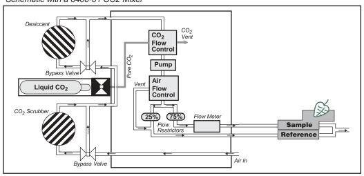
Figure 1-2. LI-6400 flow schematic, with and without a 6400-01  $CO_2$  mixer.
