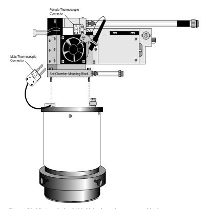
Figure 28-15. Attach the 6400-09 body to the mounting block.
