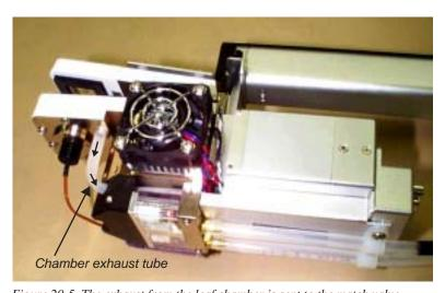
Figure 20-5. The exhaust from the leaf chamber is sent to the match valve.
