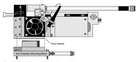
Figure 28-13. Attach the mounting block to the sensor head.
