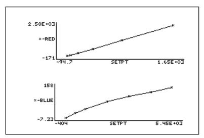
Figure 27-40. Red and Blue control signal calibration curves.
