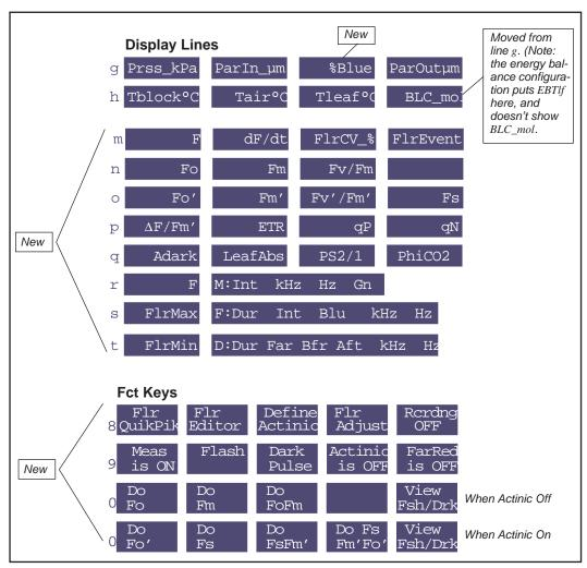
Figure 27-14. Summary of the New Measurements displays and function keys added by the default fluorescence configuration. Display explanations are in Table 27-3 on page 27-29, and the new function keys are described in Table 27-4 on page 27-32
