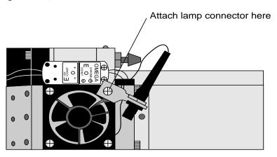
Figure 28-11. Attach the lamp connector to the fan shroud.
