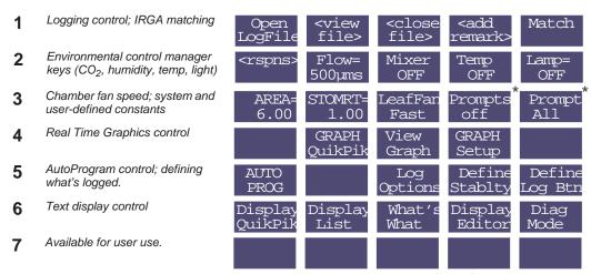
Figure 3-13. Summary of New Measurement's default function key labels.\*- keys f4 and f5 of level 3 only shows these labels when user constants are defined (described in **Prompt Control** on page 9-15).
