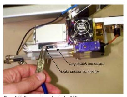
Figure 2-11. Disconnecting the in-chamber PAR sensor connector.
