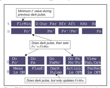
Figure 27-20. A dark pulse is triggered by either of two function keys.
