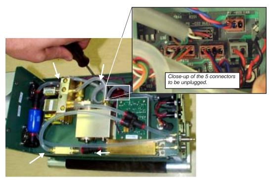
Figure 19-11. The underside of the console, showing the connector well from which all connectors should be unplugged, and the 4 screws that should be removed that hold the board assembly in place.
