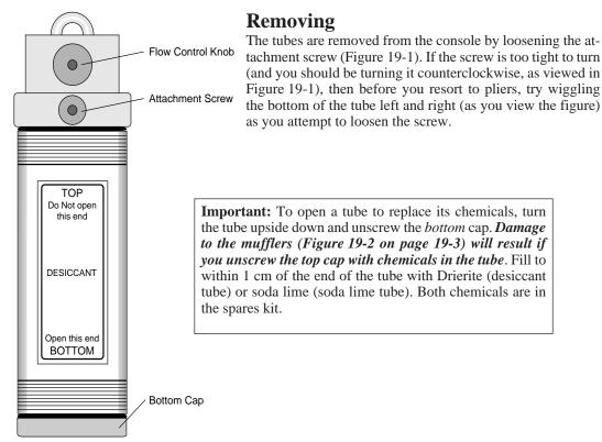
Figure 19-1. A chemical tube. The only difference between the soda lime tube and the desiccant tube is the label.
