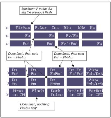
Figure 27-18. A saturating pulse (flash) can be triggered with any of these three function keys. They only differ in how the maximal fluorescence value is used.
