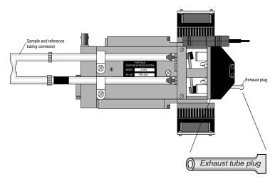
Figure 28-16. Insert exhaust plug, and sample and reference tube junction as shown.
