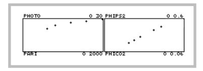
Figure 27-34. Typical light curve real time graphics. The program does light from high to low, so the light curve (left) will develop from right to left, while the PhiPS2-PhiCO2 plot (right) will develop from left to right.
