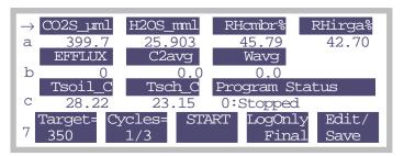
Figure 28-24. New Measurements with the soil flux configuration. Function key level 7 has most of the controls.
