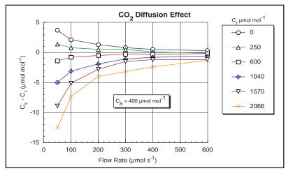
Figure 4-10.  $CO_2$  diffusion into a closed, empty LI-6400 chamber with black neoprene gaskets as a function of flow rate, for various reference concentrations  $C_r$   $C_a$  (ambient  $CO_2$ ) was 400  $\mu$ mol mol<sup>-1</sup>. Diffusion effects are highest at low flow rates and large gradients. The lines in the figure connect data of common  $C_r$
