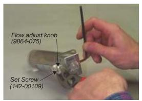
Use a 5/32 hex key to hold the flow adjust bolt, and loosen the flow adjust knob with channel lock pliers. (Turn the nut toward SCRUB to loosen.) Remove the nut and white washer that is beneath it.
