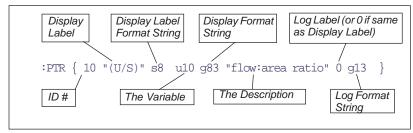
Figure 26-5. The elements of each :PTR array that make up userList[].
