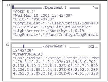
Figure 3-47. Viewing a file "as stored". a) This is the header information at the top of the file. b) After pressing **pgdn**, the rest of the file is shown. An explanation of the top line banner in each figure is given in Figure 5-1 on page 5-3.
