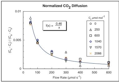
Figure 4-11. Data from Figure 4-10 normalized by the  $CO_2$  gradient,  $(C_a - C_s)$ .
