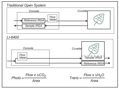
Figure 1-1. In an open system, photosynthesis and transpiration are computed from the differences in  $CO_2$  and  $H_2O$  between in-chamber conditions and prechamber conditions. The equations are given in **Equation Summary** on page 1-7.
