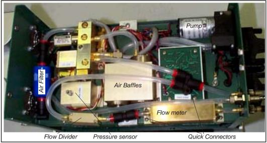
Figure 20-13. Bottom view of the console with the cover removed.
