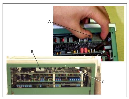
*Figure 19-10. The keyboard (A), display (B), and backlight (C) connectors.*
