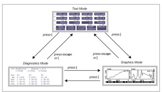
Figure 3-12. Getting around in New Measurements between the three display modes.] is the right square bracket key, and [ is the left square bracket key.
