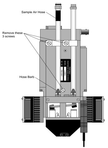
Figure 28-7. Preparing to remove the bottom plate.
