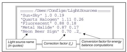
Figure 18-21. Each entry in the list source list needs a quoted name, an actinity correction factor, and a conversion factor (used only for energy balance computations).
