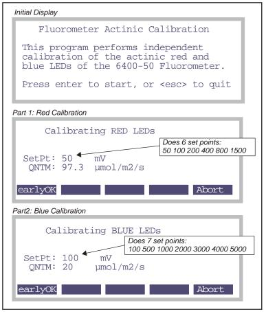
Figure 27-39. The "\_LED Source - Calibrate" program in the Calibration Menu.
