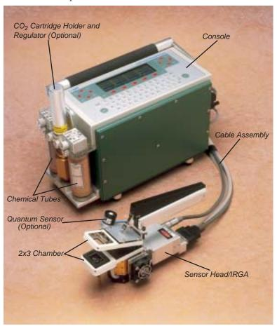
Figure 1-5. The LI-6400 Portable Photosynthesis System.
