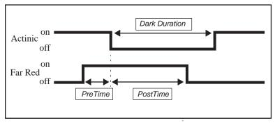
Figure 27-19. Illustration of the timing parameters for a dark pulse. The far red LED comes on PreTime seconds before the actinic light goes off, and remains on for PostTime seconds after. The actinic is off for DarkDuration seconds.
