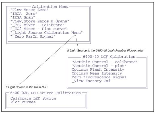
Figure 3-8. The Calib Menu. The light source calibration sub menu depends on what the light source ("Light Source Control" in the Config Menu) is currently set to.
