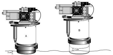
Figure 28-28. Measuring the insertion depth, <u>InsDepth</u>
