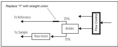
Figure 4-16. To achieve flow control down to zero, replace the T downstream of the diverter with a straight union.
