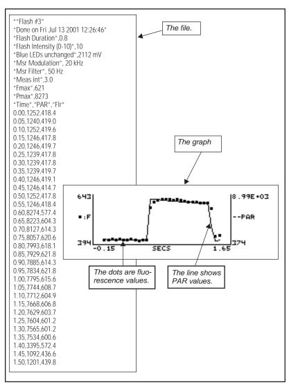
Figure 27-22. A single intensity saturating flash, graphed and stored.
