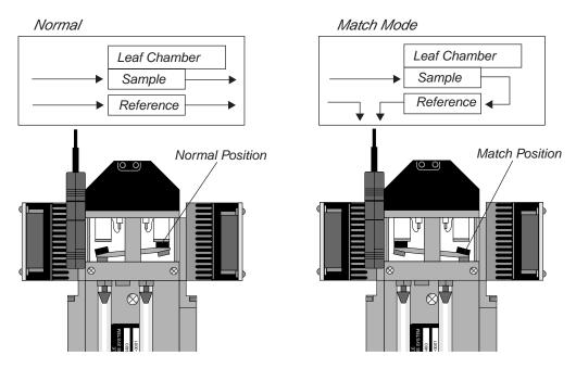
Figure 4-2. The match valve puts exhaust air from the sample cell into the reference cell, allowing both cells to be matched without altering conditions in the leaf chamber.
