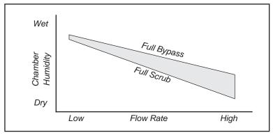
Figure 7-8. The operating envelope is determined by the transpiration from the leaf. To maintain any given humidity, a combination of flow rate and desiccant knob settings might achieve it. Typically, the knob remains fixed, and the flow is adjusted automatically.
