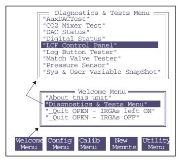
Figure 27-50. Navigating to the LCF Control Panel program from OPEN's main screen function keys.
