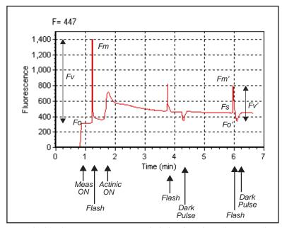
Figure 27-31. Fluorescence parameters of a light-adapted sample upon application of a saturating flash, followed by a dark period with far-red light.
