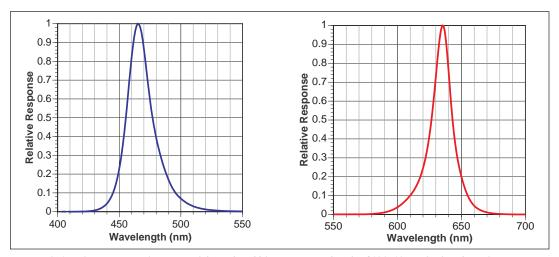
Figure 8-4. Relative spectral outputs of the red and blue LEDs used in the 6400-40 Leaf Chamber Fluorometer.
