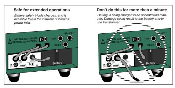
Figure 19-8. Avoid extended (more than a minute) operations with a battery and one of the AC module's plugs connected to the console. In this configuration, you will be providing uncontrolled charging of the battery, which could damage the battery and/or the transformer.
