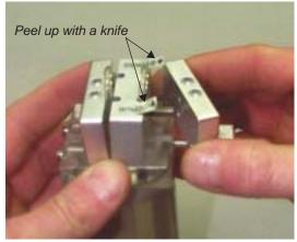
You'll have to peel the ends of the SCRUB and BY-PASS stickers up with a knife, then the two loose pieces of the assembly can be removed.
