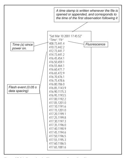
Figure 27-24. Example of a Fluorescence Recording file.
