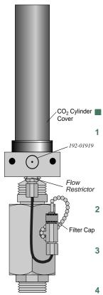
Figure 19-34. Location of oil filter cap.
