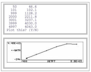
Figure 18-18. The LED source calibration data is displayed, and you are given a chance to plot the graph.
