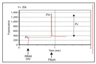
Figure 27-27. Fluorescence parameters of a dark-adapted plant upon application of a saturation flash.
