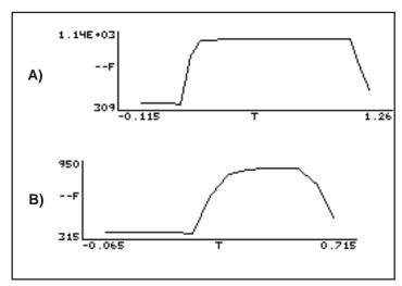
Figure 27-28. A) Example of a good saturation flash: flash length and intensity are appropriate for this leaf material (philodendron dark-adapted for 20 minutes). B) Example of a poor saturation flash: flash length was too short and intensity too small.
