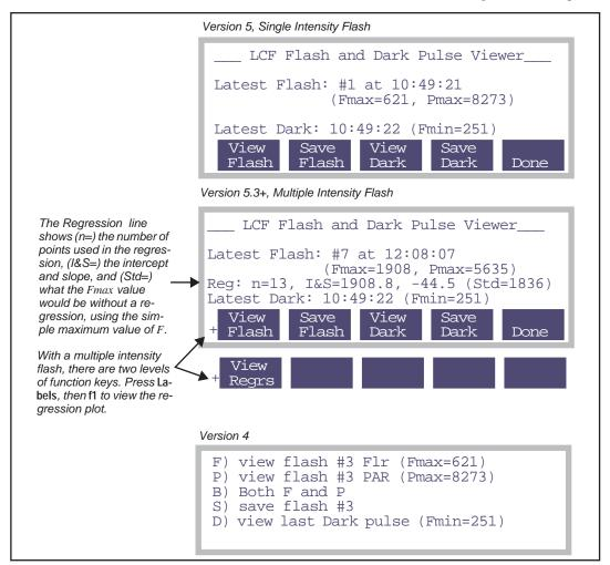
Figure 27-21. The View Flash/Dark screen for the two software versions.
