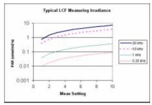
Figure 27-37. Typical measuring beam quantum irradiance values for the 6400-40 LCF, as a function of measuring beam setting and modulation rate. These data were measured with an LI-1800 Spectroradiometer and an integrating sphere.
