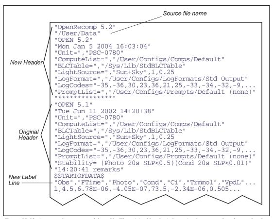
Figure 13-12. An example recomputed data file. The original header information is preserved, and a new header written before it containing the configuration used for the recomputation. The label line will reflect the log format file used for the recompute.
