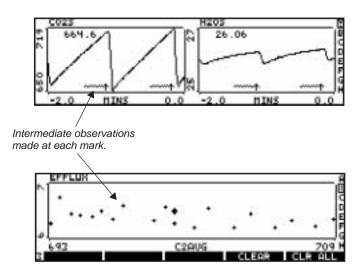
Figure 28-30. Sample of the Real Time Graphs for soil flux measurements.
