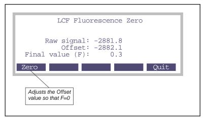
Figure 27-48. The fluorescence signal zeroing routine.
