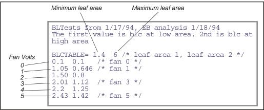
Figure 14-3. Listing of the boundary layer lookup table "/Sys/Lib/StdBLCTable". The data follows the BLCTABLE= string, and two values are expected in that line: the minimum leaf area, and the maximum leaf area. Following this comes 6 lines, one for each fan speed voltage (0 to 5). On each line is a pair of values: the one-sided boundary layer conductance for the low area, and the boundary layer conductance for the high area. The values have units of mol  $m^{-2}$  s<sup>-1</sup>.
