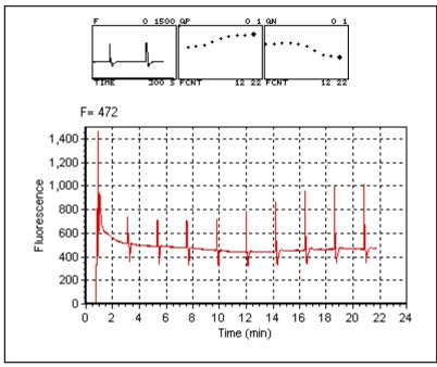
Figure 27-33. Sample results from Experiment 4. The upper graphs are the real time graphics images produced on the LI-6400 console, and show the last 300 seconds of F, and QP and QN as a function of flash count (FCNT). The lower plot showing the trace of F for the entire experiment illustrates a use of fluorescence recording (f5 level 8).
